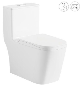
ET-2071 ONE-PIECE TOILET 4 Super Siphonic 700×360×760mm S-trap 300mm
