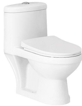
ET-001 ONE-PIECE TOILET Washdown 510×310×520mm P-trap 180mm S-trap 300mm
