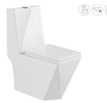
ET-2011 ONE-PIECE TOILET Siphonic/Washdown 680×370×790mm P-trap 180mm S-trap 250/300mm
