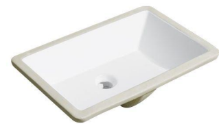
ET-2134 UNDER COUNTER BASIN Size: 530×340×190mm Inside diameter: 470×290mm
