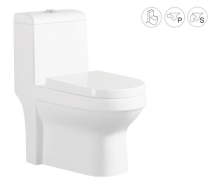
ET-2062 ONE-PIECE TOILET Siphonic/Washdown 695×366×805mm P-trap 180mm S-trap 250/300mm
