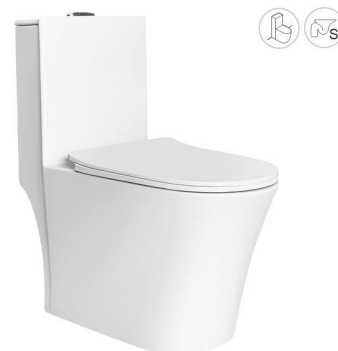
ET-2073 ONE-PIECE TOILET 4 Super Siphonic 680×370×765mm S-trap 300mm
