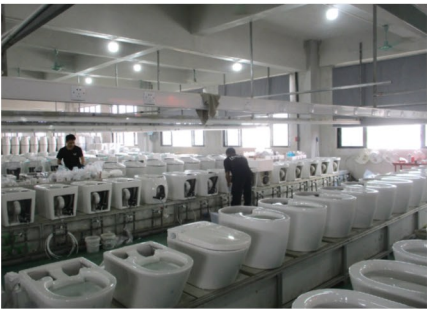
Complete installation and function testing
