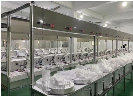
Function testing of smart seat cover
